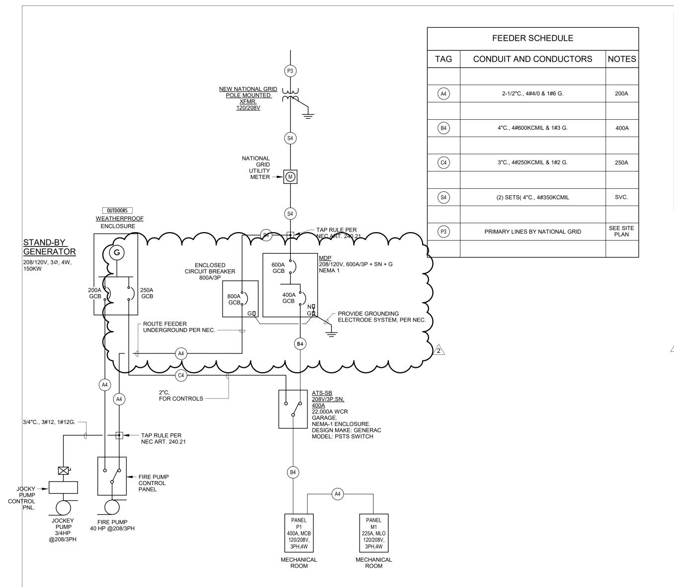
$\underbrace{1}_{\text{N.T.S.}} \underbrace{\text{ONE-LINE DIAGRAM}}_{\text{N.T.S.}}$
